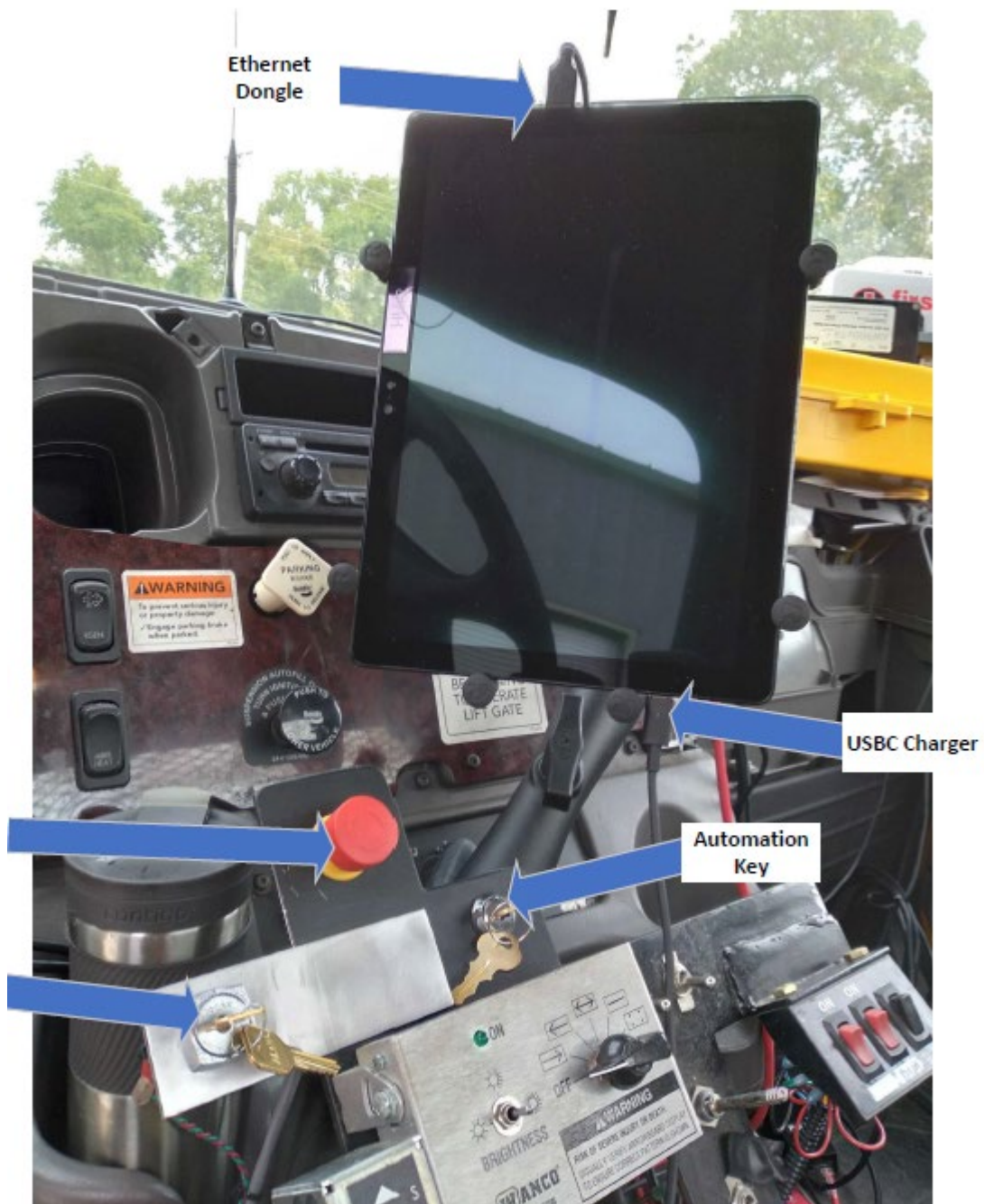
Image 6: Automation keys and Emergency Stop
