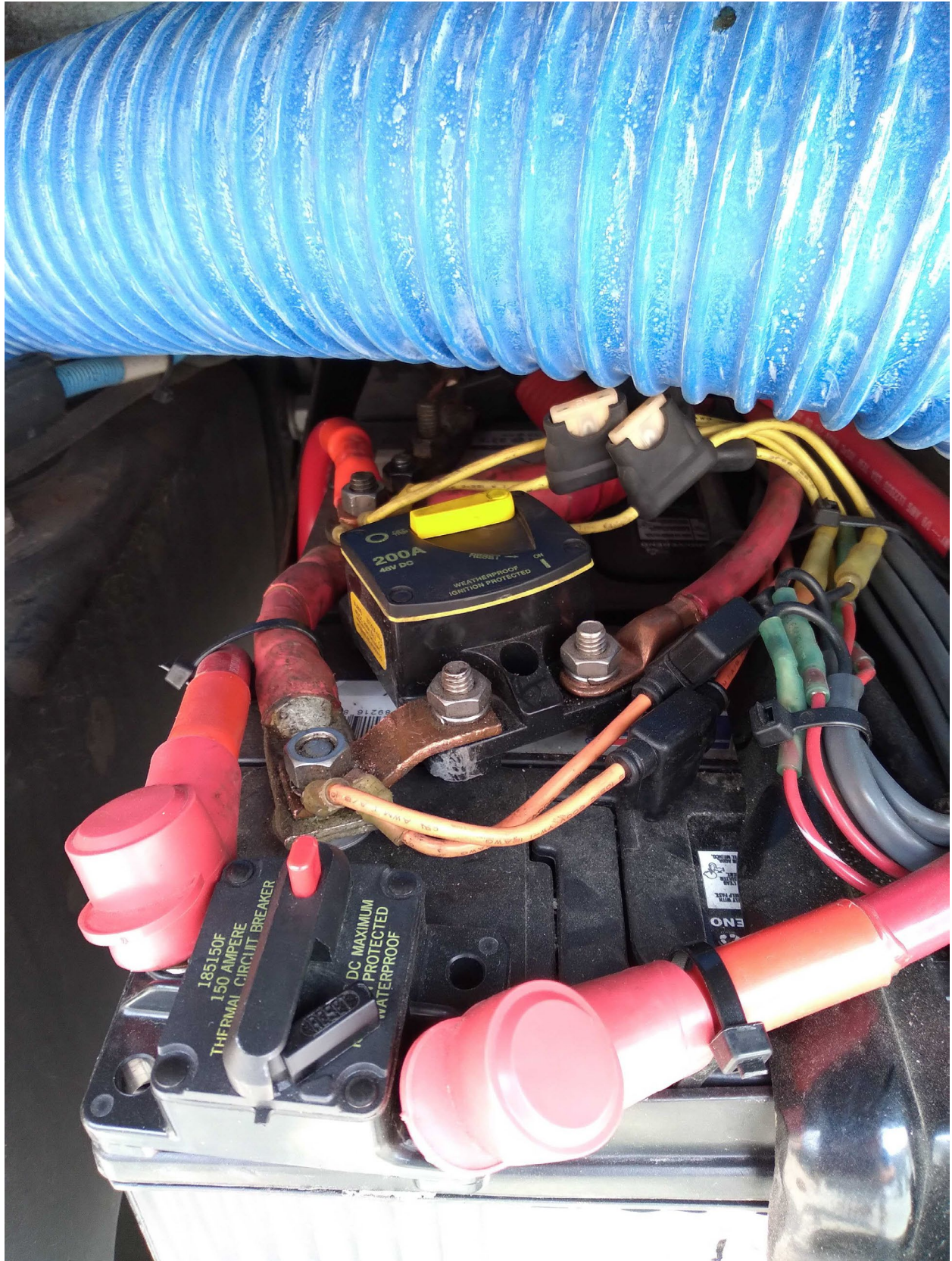
Image 3: Battery Breakers (2)
